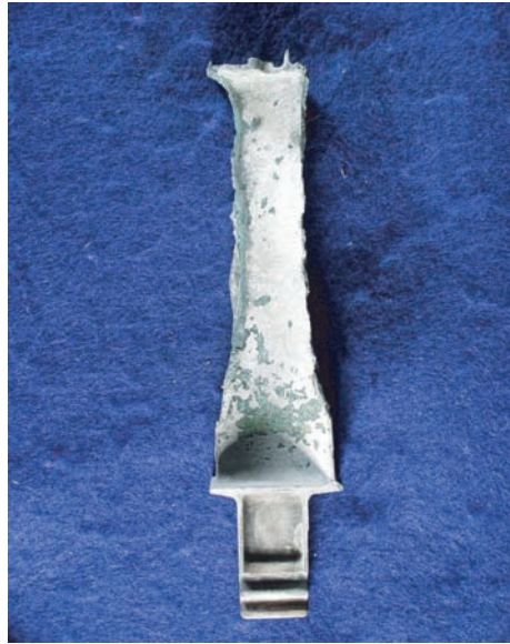
Fig. 28 Severe attack of an aeroderivative gas turbine blade by hot corrosion. See the article "Corrosion of Industrial Gas Turbines" in this Volume.
