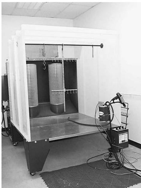
Fig. 11 Powder coating spray booth at a naval air depot
