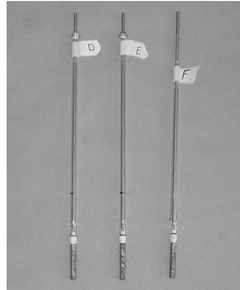
Fig. 9 Soil corrosion electrodes used in the soil test cell in Fig. 8.
