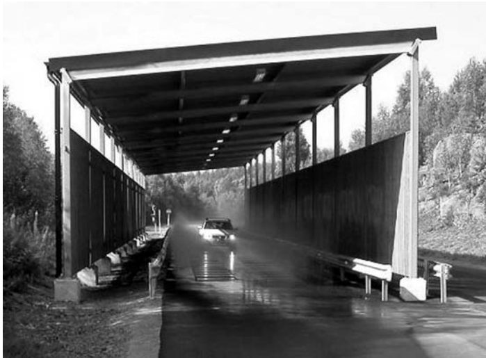
Fig. 1 Proving ground highway simulating splash/spray during high wintertime conditions with deicing salt use. Note the shallow splash groves in the highway.
