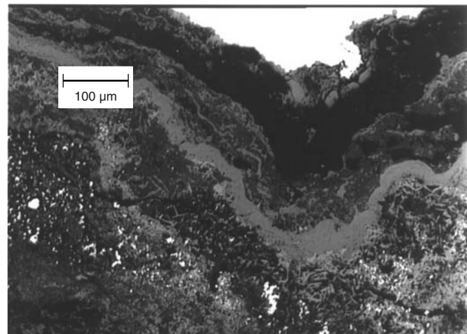
Fig. 4 Hot side deposit in the vicinity of the failure displays several layers and waterside oxidation/corrosion. Some layers are dense, while others are very porous. One layer displayed needlelike, fibrous oxides. Another layer contains a number of particles of copper metal. Original magnification 210\times
