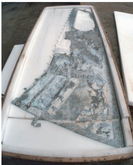
Fig. 15 Aluminum horizontal skin exhibiting extensive water-induced corrosion due to improper packaging and preservation during shipment from the manufacturer. Courtesy of S. Bevan, Naval Air Depot, Jacksonville. See the article "U.S. Navy Aircraft Corrosion" in this Volume.
