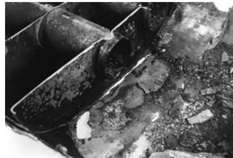
Fig. 24 Internal view of muffler with 14,500 km (9,000 miles) of service. Condensate galvanic corrosion between the 409 stainless baffles and ALT1 shell has destroyed the wrap.
