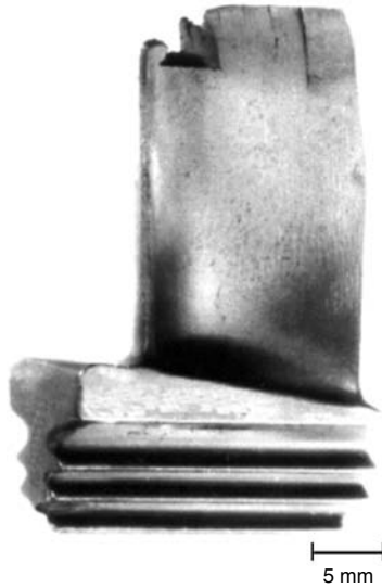
Fig. 9 Tip cracking of a directionally solidified MAR-M-246 turbine blade
