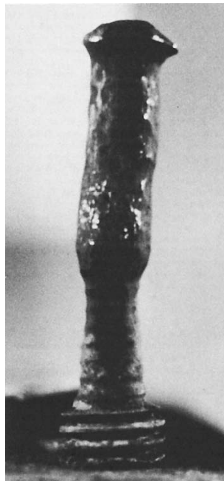
Fig. 2 Monel 400 bonnet bolt extensively corroded by chlorine gas trapped beneath ice covering a valve in liquid chlorine service
