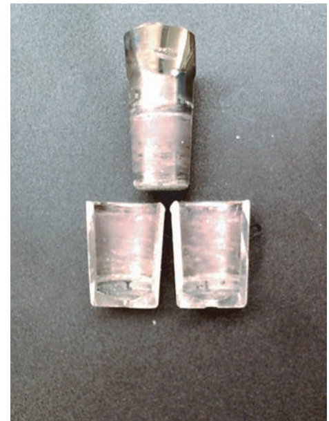
Fig. 40 Light photographs of modular tapers from prostheses showing evidence of corrosion. Retrieved Ti-6Al-4V neck and Ti-6Al-4V "thimble" (sectioned in half) used to attach a ceramic head to the femoral stem. Two modular interfaces are established in this design, one comprising the titanium-titanium junction and the other the titanium-ceramic junction. Note that the interface regions are highly corroded on both titanium interfaces, and a purple color was present (indicative of Ti 3+ ions). Also found at these interfaces is evidence of titanium-phosphate particles, which indicate that the pH had dropped below 1 inside the taper. See the article "Mechanically Assisted Corrosion of Metallic Biomaterials" in this Volume.
