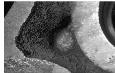
Fig. 5 Pitting corrosion in aluminum cylinder head port
