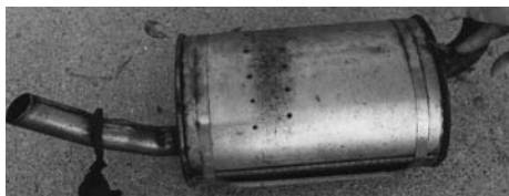
Fig. 9 T439 muffler shell after 106,500 km (66,000 miles) of driving. Cosmetic superficial pitting seen in band above a tuning chamber area that saw higher temperatures and heat tinting
