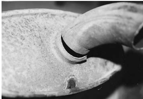
Fig. 23 Galvanic corrosion when mixing muffler materials. Aluminum sacrifices itself to protect the 409 stainless steel, exposing the carbon steel substrate.
