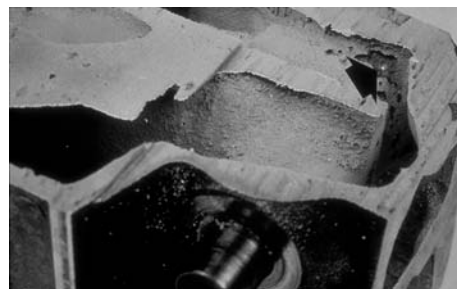
Fig. 8 Nucleate boiling-induced cavitation corrosion caused perforation at the exhaust valve port of this aluminum cylinder head.
