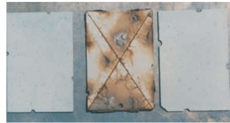
Fig. 8 Scribed, sealed and painted thermal spray coatings on steel substrates compared to a scribed, painted steel panel after 42 months of severe marine atmospheric exposure. See the article "Corrosion of Metallic Coatings" in this Volume.
