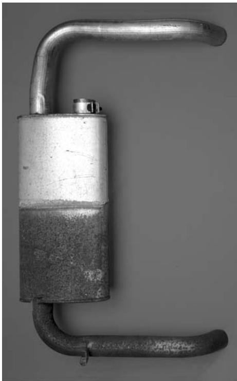
Fig. 26 Muffler with wrap and heads half made of bare 409 (bottom portion) and half of AL409 (top portion) and test driven 27,400 km (17,000 miles). Bare 409 gas metal arc weld and band of bare 409 adjacent to the weld galvanically protected by aluminum coating
