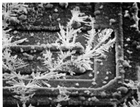
Fig. 4 Example of dendrite growth on the surface of an integrated circuit, in this case, silver, which is no longer used. Source: Ref 42
