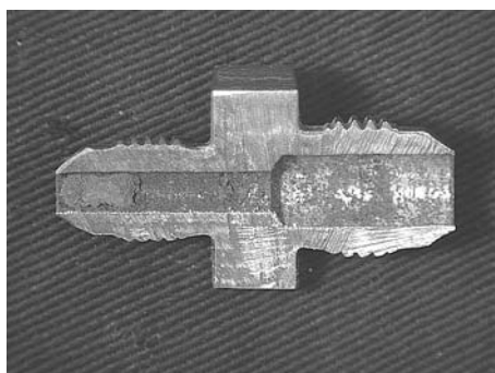
Fig. 19 High-temperature corrosion of a 300 series stainless steel union fitting within an EA-6B canopy ejection system. Courtesy of J. Benfer, Naval Air Depot—Jacksonville
