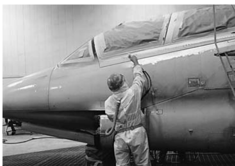
Fig. 9 Application of nonchromated waterborne epoxy primer to a T-2 aircraft at a naval air depot
