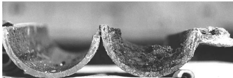
Fig. 2 Side view of tube sample reveals that hot side deposits are as much as 25 mm (1.0 in.) thick. Relatively little deposition was present on the cold side
