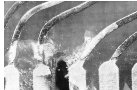
Fig. 4 White corrosion products on tin-coated circuits and galvanic corrosion between the gold-tin contact/circuit interface resulting from a coffee spill
