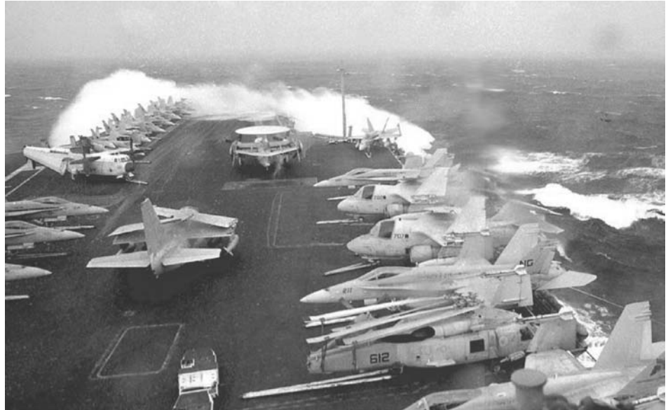
Fig. 8 Naval aircraft carrier flight deck environment containing salt fog, hydrocarbons, and engine exhaust gases such as \text{SO}_2 , \text{NO}_x , and so forth
