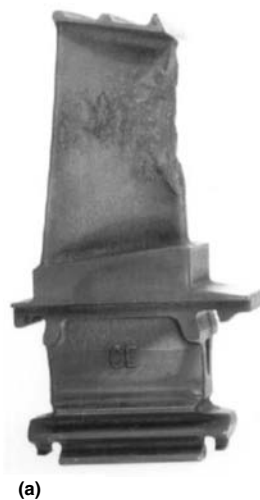
Fig. 8 Examples of engine component surface damage. (a) Evidence of hot corrosion damage on the pressure side of a MAR-M-246 turbine blade. (b) Metallographic section across the airfoil of the MAR-M-246 blade, showing evidence of hot corrosion damage penetrating the leading edge (B) right through to the internal cooling passage (A)
