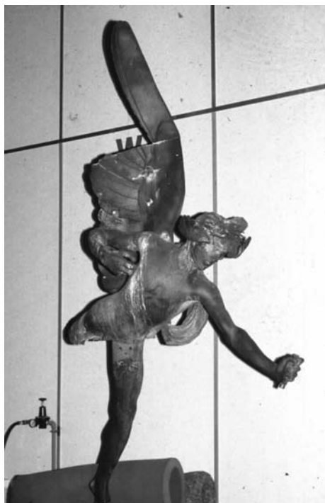
Fig. 8 Cast aluminum statue of Eros by Alfred Gilbert (cast 1929) in Liverpool, England, before treatment. The damage to wings was caused by corrosion of internal iron armatures. Courtesy of Martin Cooper, National Museums Liverpool. Photograph circa 1994
