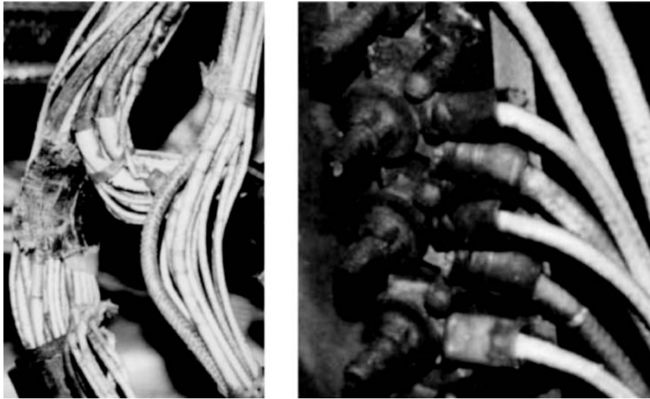
Fig. 13 Wiring insulation cracks (left) and corroded terminals on a C130 (right)
