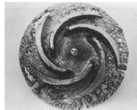
Fig. 7 Erosion-corrosion of ACI CN-7M stainless steel pump components that pumped hot H_2SO_4 with some solids present. Note the grooves, gullies, waves, and valleys common to erosion-corrosion damage. Courtesy of A.R. Wilfley & Sons, Inc., Pump Division
