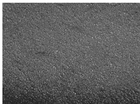
Fig. 12 Class 1 rouge that is transported from other locations and deposited on the stainless steel surface. It is amorphous in structure, and the color varies from orange to red. The primary mineral form is hematite, \text{Fe}_2\text{O}_3 . SEM; original magnification 450 \times
