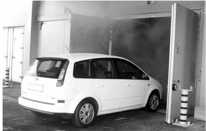
Fig. 2 Garaging of a test car in a proving ground humidity chamber after a daily test track driving sequence
