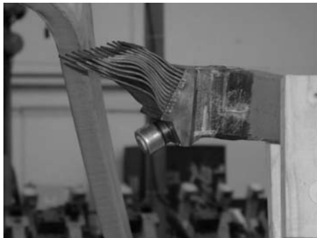
Fig. 3 End of a water-cooled coil. This "bottle clip," made of copper, allows the coil to be electrically connected to the next coil by means of the laminated flexible connector and also provides a means of cooling water to pass through this coil and out the machine.
