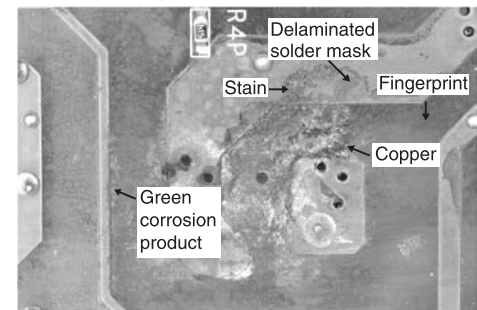
Fig. 24 Copper migration and corrosion on surface of failed printed circuit board
