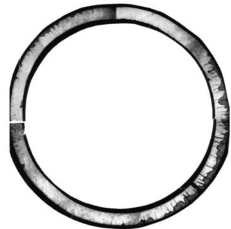
Fig. 18 An example of severe intergranular attack/intergranular stress-corrosion cracking (IGA/IGSCC) at a tube support location. Source: Ref 80
