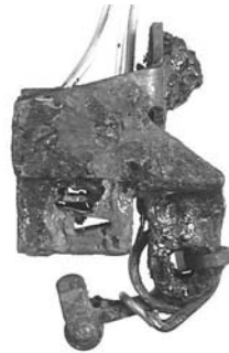
Fig. 16 Slat gearbox limit switch for EA-6B aircraft following ASTM B 117 neutral salt-spray corrosion testing without MIL-L-87177 corrosion-inhibiting lubricant. Courtesy of J. Benfer, Naval Air Depot—Jacksonville
