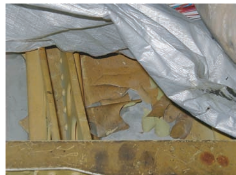
Fig. 14 Loss of paint adhesion caused by silicone contamination. See the article "U.S. Navy Aircraft Corrosion" in this Volume.
