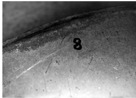
Fig. 19 Muffler with 27,400 km (17,000 miles) of service and AL409 wrap and end cap. Condensate leakage through the rolled head has attacked the aluminum coating.
