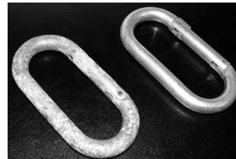
Fig. 10 The carabiner in the foreground was found in a damp cave in upstate New York. A similar aluminum alloy carabiner is shown for comparison. In addition to white corrosion product generally present over all surfaces, there is red rust at the hinge and catch pins and the carabiner is frozen in the closed position. Courtesy of Lorrie Krebs, Anderson Materials Evaluation, Inc.
