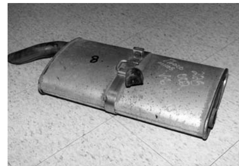
Fig. 25 Muffler with AL409 wrap and bare stainless belly band and end cap (right side of image). After 27,400 km (17,000 miles) of driving service, the band and muffler end plate have led to galvanic attack on the aluminum coating of the wrap.
