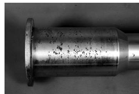
Fig. 1 Pitting of 25 µm (1.0 mil) chromium plating on a steel pin used to join the lower carriage to the trails on a towed howitzer. The chromium plating should be twice this thickness to serve as an effective barrier coating for this application
