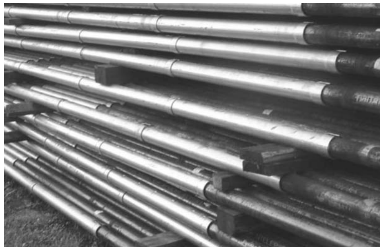
Fig. 7 Carbon steel superheater tubes protected by metallic tube shields awaiting installation at one waste-to-energy plant
