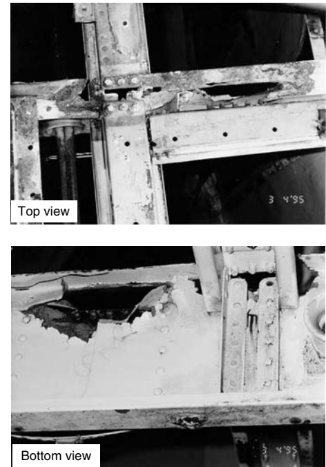
Fig. 15 Aluminum floor structure corrosion in a 767 at forward entry door
