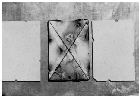
Fig. 3 Comparison of scribed, sealed, and painted thermal spray coatings on steel substrates to a scribed painted steel panel after 42 months of severe marine atmospheric exposure. (a) Flame-sprayed aluminum on steel, sealed/painted. (b) Painted steel panel (one coat MIL P24441 F150 primer followed by one coat of formula 150 and one coat formula 151). (c) Arc-sprayed aluminum on steel, sealed/painted
