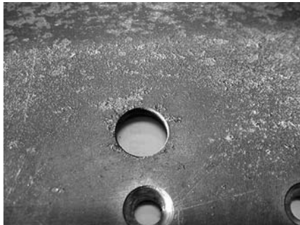
Fig. 12 Corrosion of a nickel-plated aluminum mounting bracket for AV-8 aircraft due to atmospheric exposure. Courtesy of J. Whitfield, Naval Air Depot—Cherry Point
