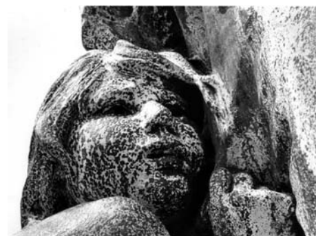
Fig. 5 Detail of severe pitting on a child's face in the 1887 bronze statue Stone Age in America by John J. Boyle located in Philadelphia. Courtesy of the Fairmount Park Art Association. Photograph by Franko Khoury © 1983
