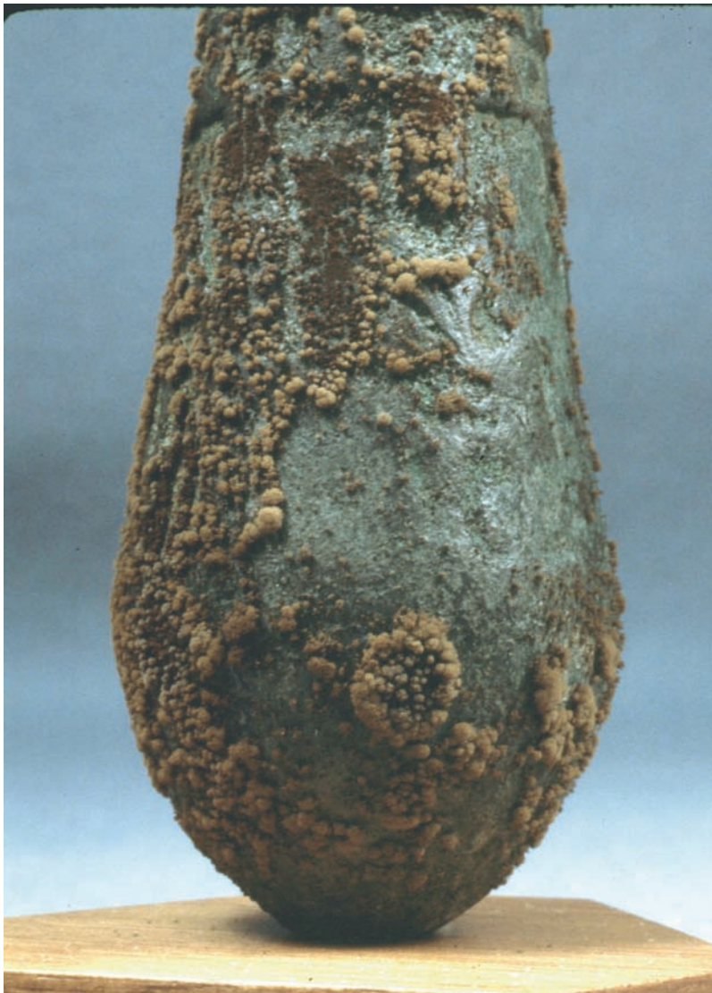
Fig. 20 Velvetlike corrosion growths on the surface of an ancient copper alloy vessel. The subtle form of the object is all but obscured by corrosion growths. See the article "Corrosion of Metal Artifacts and Works of Art in Museum and Collection Environments" in this Volume.
