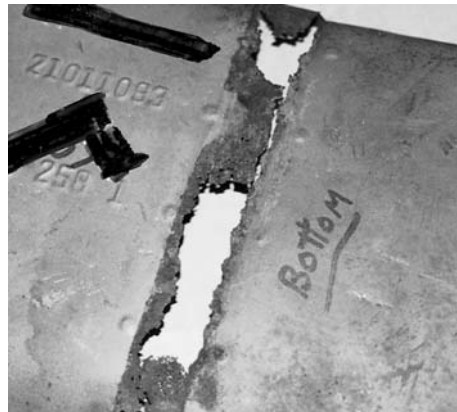
Fig. 20 Crevice corrosion of a 409 muffler shell under a belly band (removed from photo) on a vehicle driven 114,500 km (71,000 miles) in Montreal, Canada.
