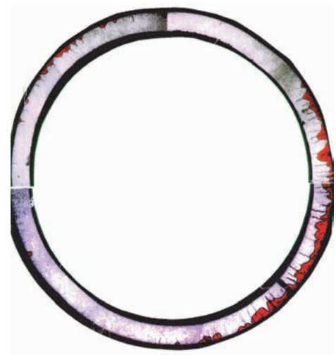
Fig. 39 An example of severe intergranular attack/intergranular stress-corrosion cracking at a tube support location. See the article "Corrosion in Pressurized Water Reactors" in this Volume.
