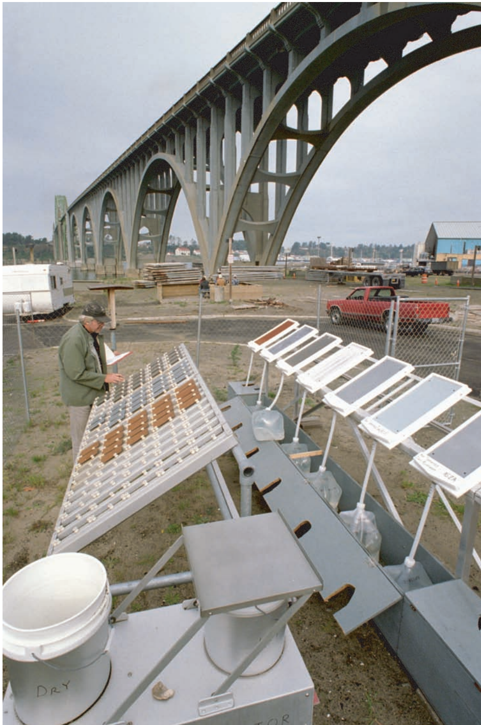
Fig. 7 Marine atmospheric corrosion and precipitation runoff test site at Newport, OR. See the article "Simulated Service Testing in the Atmosphere" in ASM Handbook Volume 13A of this series.
