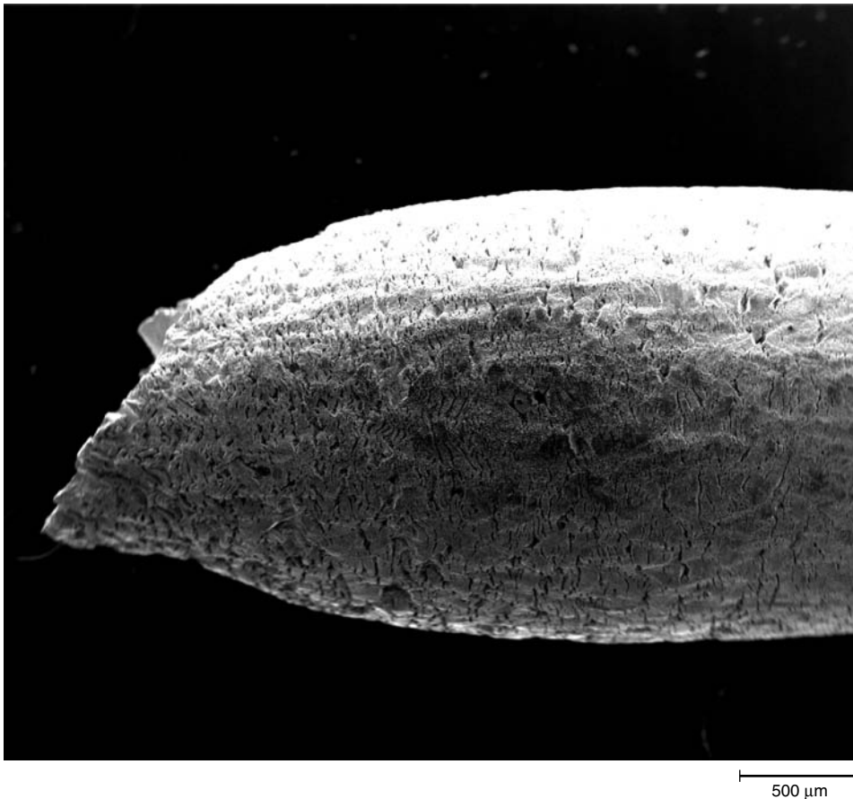
Fig. 8 Mill annealed alloy 22 specimen ARC22-032 strained in simulated corrosion water at 50 °C (120 °F) and +400 mV applied potential. Negligible amount of secondary cracking and obvious necking is observed. Original magnification: 70×
