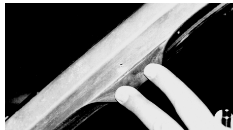
Fig. 3 Crevice corrosion under a windshield gasket
