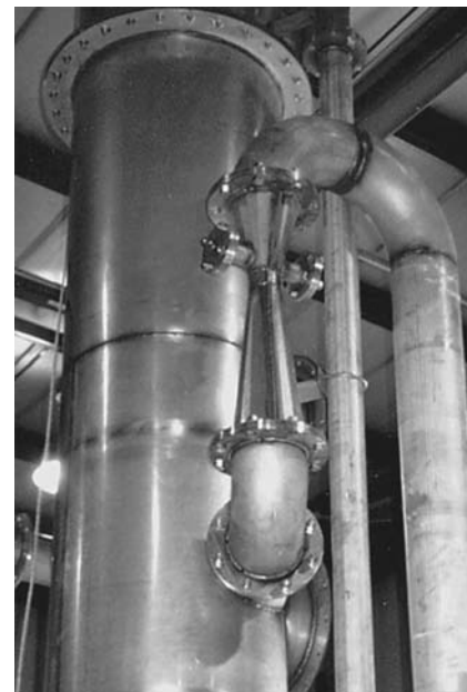
Fig. 3 A stainless steel venturi tube scrubber separator. Courtesy of Branch Environmental Corporation
