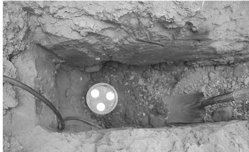
Fig. 11 Three-electrode soil corrosivity probe
