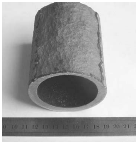
Fig. 1 The overlay cladding, approximately 2 mm (80 mils) thick of alloy 625 (UNS N06625) overlay superheater tube, was corroded away in 15 months in a waste-to-energy boiler.
