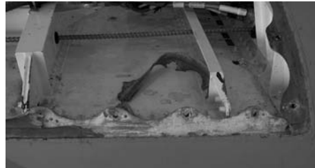
Fig. 13 Galvanic corrosion of F/A-18 aircraft dorsal scallops resulting from composite doors attached to aluminum substructure with titanium and steel fasteners in the presence of moisture. Courtesy of S. Long, Naval Air Depot—North Island
