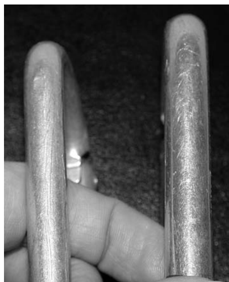
Fig. 9 One way to reduce weight when climbing is to use carabiners with smaller cross sections. The trade-off is in the load-bearing capacity rating. Courtesy of Lorrie Krebs, Anderson Materials Evaluation, Inc.
