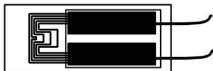
Fig. 5 Thin film electrical resistance probe. Source: Ref 10
