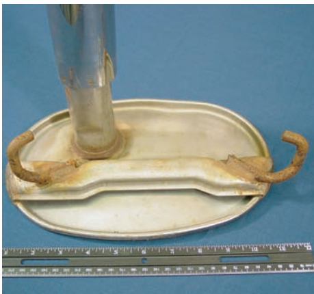
Fig. 23 Galvanic corrosion of solid carbon steel hanger rods after 1.5 years of driving service in the salt belt. Muffler end plate and sheet metal hanger are 18Cr-Cb. See the article "Automotive Exhaust System Corrosion" in this Volume.
