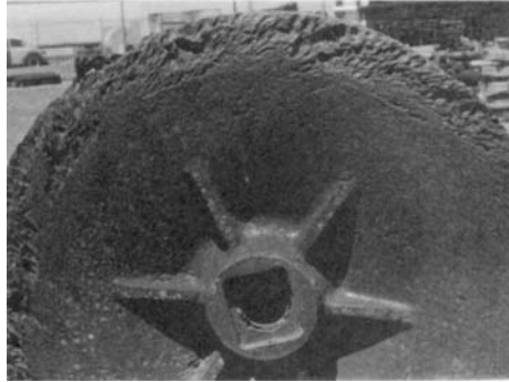
Fig. 8 Erosion-corrosion of an abrasion-resistant iron pump runner used to pump 30% iron tailings in a fluid with a pH of 11.2. This runner had a service life of approximately 3 months. Note that most of the damage is on the outer peripheral area of the runner where fluid velocity is the highest. Courtesy of A.R. Wilfley & Sons, Inc., Pump Division
