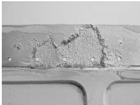
Fig. 15 Corrosion damage of a T-45 aircraft access panel. Corrosion initiates at and beneath electromagnetic interference (EMI) fingers (removed) needed to control the EMI. Courtesy of J. Benfer, Naval Air Depot—Jacksonville
