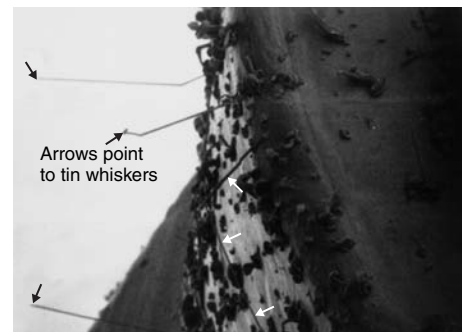
Fig. 32 Scanning electron micrograph of tin whiskers on base of insulated standoff terminal
