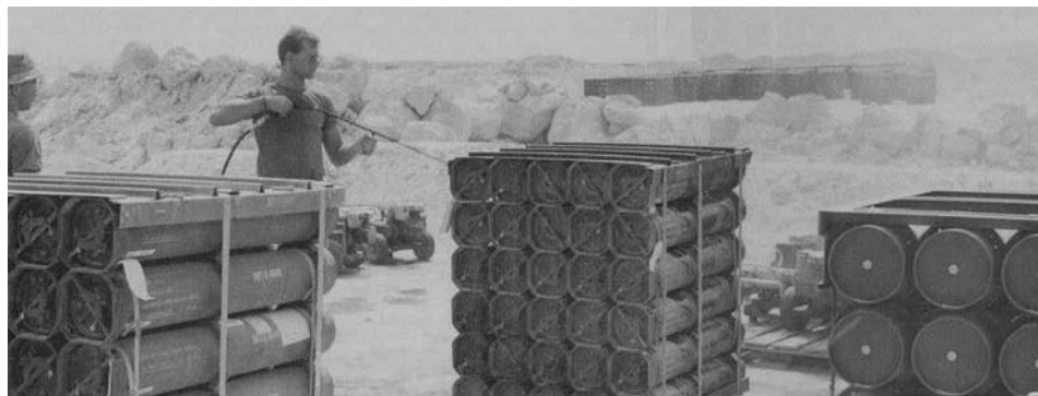
Fig. 9 Pressure washing of ammunition containers. Source: Ref 6
