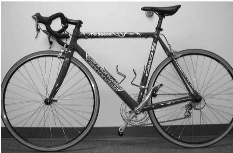
Fig. 2 This Cannondale composite bicycle has an aluminum frame and a carbon fiber fork, resulting in a more corrosion-resistant bicycle than the more common (worldwide) steel frames. However, important components such as chains, axles, and bearings are still commonly made of steel for strength requirements and must be maintained to prevent corrosion from forming and interfering with performance. Courtesy of Greg Welsh
