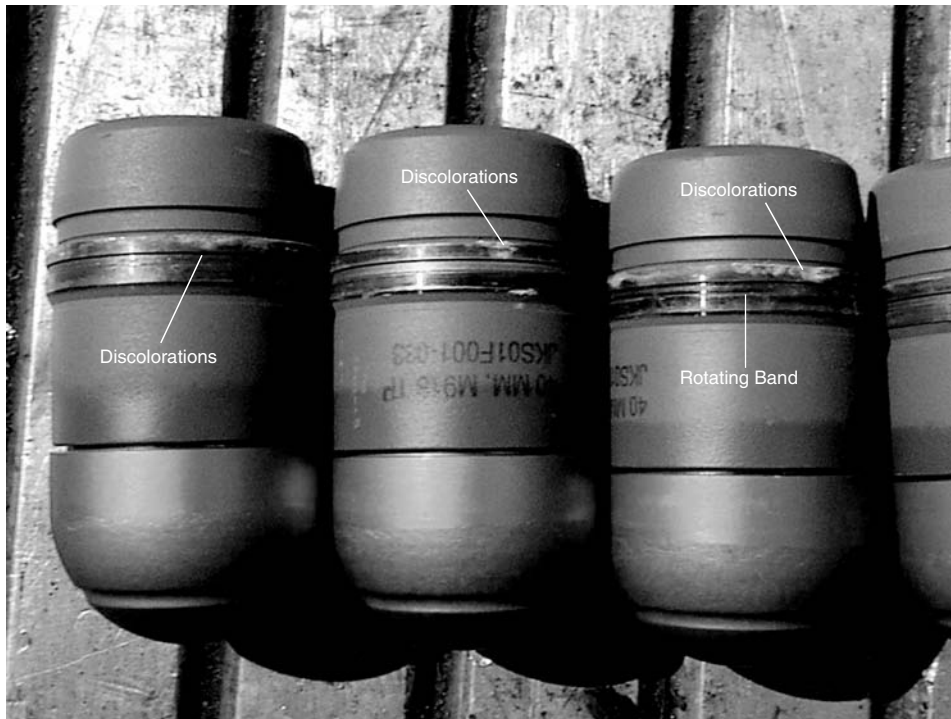
Fig. 5 Grenade body showing discoloration of copper rotating bands resulting from exposure to trapped machining lubricant. Source: Ref 4
